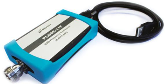
PLG signal generator creates harmonic signals with frequency tuning range from 25 MHz to 6/12/20 GHz with 1 Hz step and power tuning range from -40 to -10 dBm with 1 dB step. The output signal can be modulated by an internal or external source.
